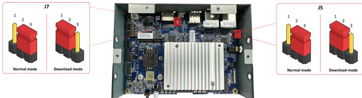
OS image jumpers diagram
