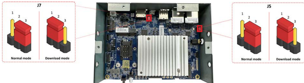
OS image jumpers diagram
