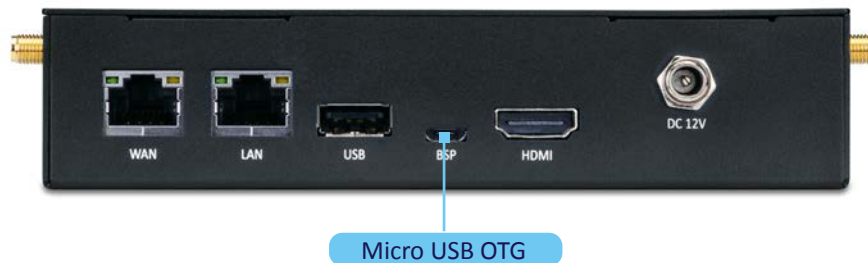
Micro USB 2.0 port diagram
